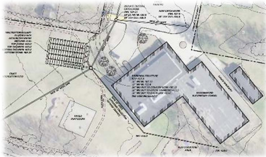
Figure 3: Vignette from the 30% concept design for the Wallingford School infiltration chamber system. The system would take drainage from the entire school area, including some of the road and residential neighborhood adjacent to the school.
